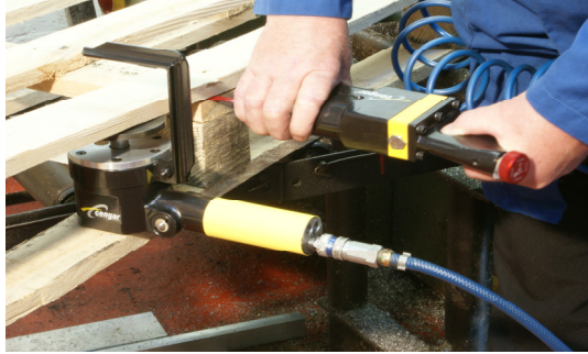
Cengar Saw and Pallet Spreader in use
