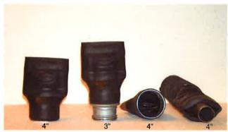
The FlexGrip nozzle is a basic oval nozzle for single exhaust pipes. The opening is sufficiently narrow and stiff to grip tight without any other type of activation. The upper lip is thin and flexible, whereas the lower lip is so thick that it closes the opening when not is use.
