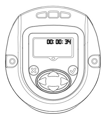
Displays Tool time in HH:MM:SS format. Press the Down key to display the tool time in HH:MM:SS format.
