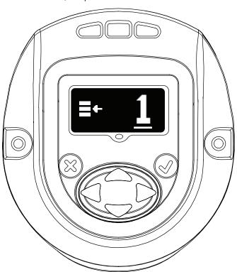
"UP" or "DOWN" key can be used to update the configuration. Pressing "ENTER" again will select the modified configuration.
