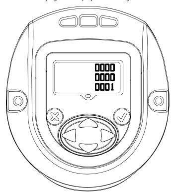
Press the Down key again to return to the Tool ID page. Pressing the right arrow from this page exits back to the password display.
