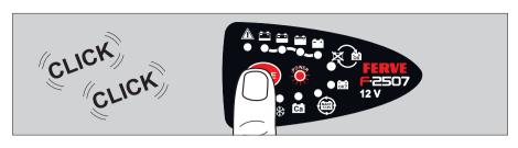
Press the MODE button until the LED turns on (flashing light).
