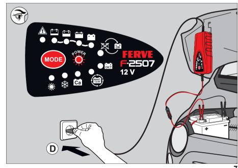
Connect the FERVE F-2507 charger to a mains supply (D). The LED POWER turns on and the charging process begins.
