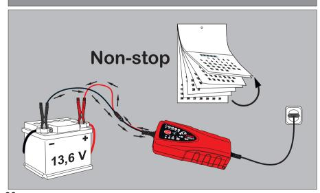
If you leave it plugged in, the FERVE F-2507 autocharge will keep the battery at a constant voltage of 13.6 V.
