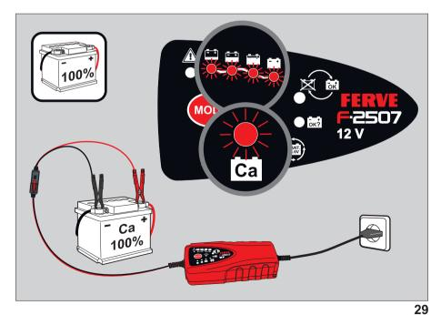
When the 4 LEDs  $\stackrel{\square}{=}$   $\stackrel{\square}{=}$  are on solidly, the battery is fully charged and the FERVE F-2507 can now be disconnected.
