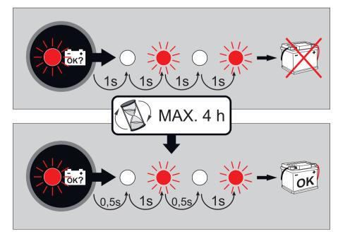
The LED flashes at intervals of 1 second. If within a period of 4 hours the flashing continues at intervals of 1 second, the battery cannot be recovered and must be replaced. The battery may have been recovered when the flashing is at intervals of 0.5 seconds (on) / 1 second (off).
