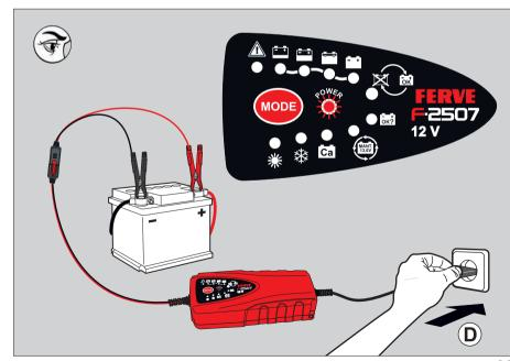
Connect the FERVE F-2507 charger to a mains supply (D). The LED POWER turns on and the charging process begins. If the LED POWER is permanently on, the battery is faulty or sulphated.
