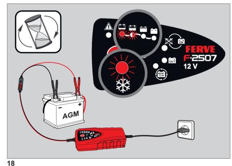
The upper four LEDs 🔛 🖼 🖼 indicate the battery's charge status and they turn on progressively as the charging proceeds.
