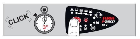
Press and hold the MODE button for 3 seconds until the LED ca turns on. The charging process starts.
