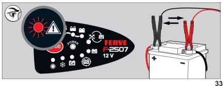
Connect the clamps to the battery in the following order: first the red clamp to the positive terminal + (A) and then the black clamp to the negative terminal - (B). Finally, connect the clamps to the charger (C).
