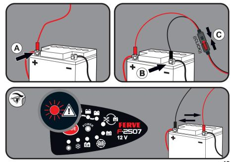
Connect the terminals to the battery terminals in the following order: first the red terminal to the positive terminal + (A) and then the black terminal to the negative terminal - (B). Finally, connect the terminals to the charger (C).
