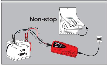
If you leave it plugged in, the FERVE F-2507 autocharge will keep the battery at 100% capacity at all times.
